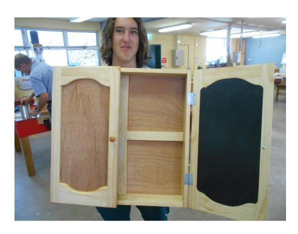
The Dartboard cabinet with a linseed oil finish. Blackboard paint has been applied to the inside of the door panels.
