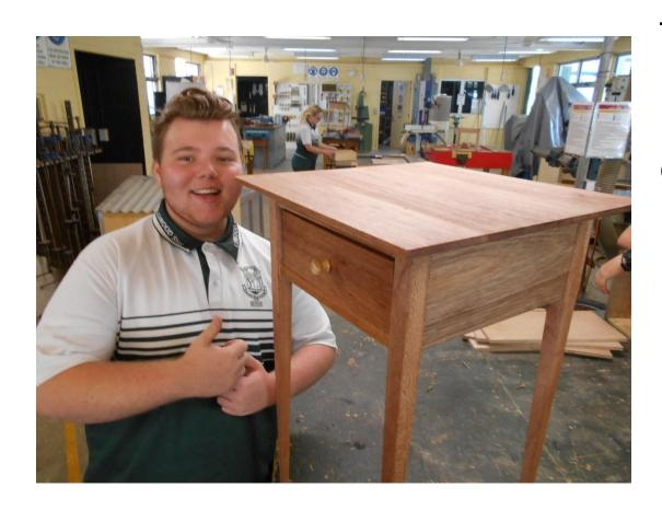
The shaker table with drawer has been finished with tung oil. This project may be replaced with the classical guitar.
